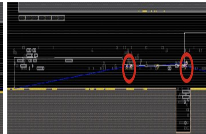
Fig 7: Proposed Solution : Buffers used on the path
